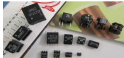
Data Coupling Transformers
